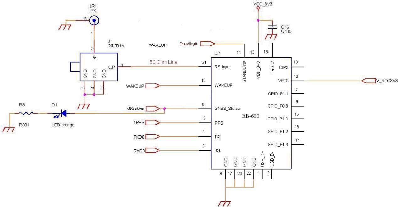
**【Note 1】** : VRTC (pin#12) could connect to 3.3V DC power supply or battery directly. (EB-600)
