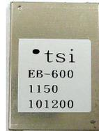
Pin locations backward compatible with TSI's EB-500, you can easily upgrade your system to latest high sensitivity GPS + Glonass receiver available in the industry.
